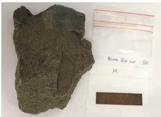
Figure 3-6. Corrosion coupon S2/M with surrounding bentonite clay.
