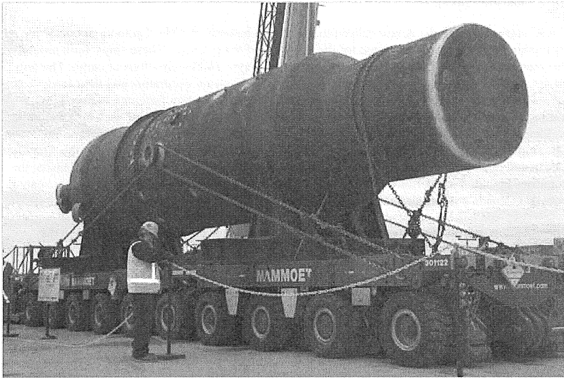
Figure 5: Steam generator loaded onto a self-propelled modular transporter
